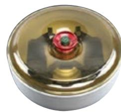
**BIOShield 720 Swinging Buckets Rotor, 90°, R<sub>max</sub> 162 mm**
