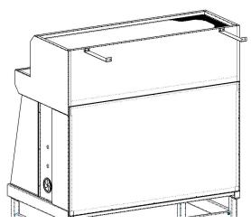
Fig. 11 Position anti-tilt anchor
