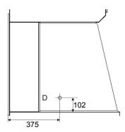
Fig. 16 Positions feed-throughs
