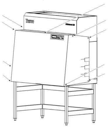
Fig. 9-3 Position of the magnetic plates
