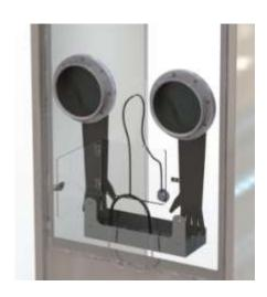
Operators side is designed with a large airtight and sealed acrylic window with two glove ports for the operator, a membrane port for stethoscope and an airtight sealed hatch for transferring samples after decontamination. Inside the test booth, accessible from the glove ports and transfer hatch, there is a usable shelf for detergents, test-kit and other necessities.
