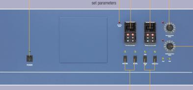
Under-temperature Safety Thermostat and Indicator Set under-temp control (alarm and light indicate under-temp condition)
