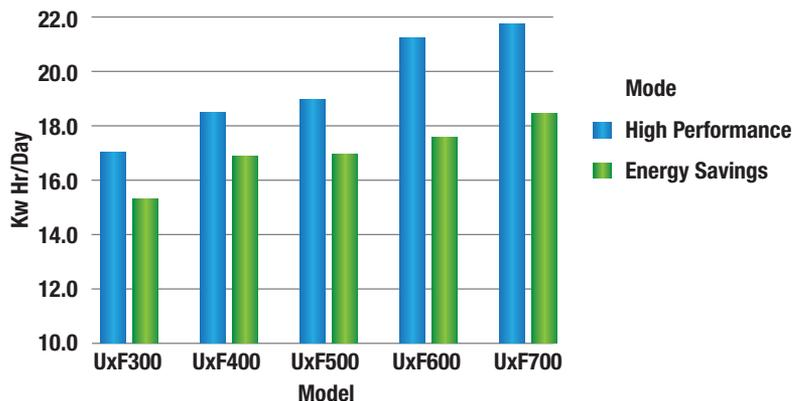
By controlling the temperature and time of the cycles, the energy savings cycle can save up to 15% while still offering tightly-controlled cabinet temperature and excellent door-opening recovery. The high-performance mode maintains the strictest cabinet temperature control.
