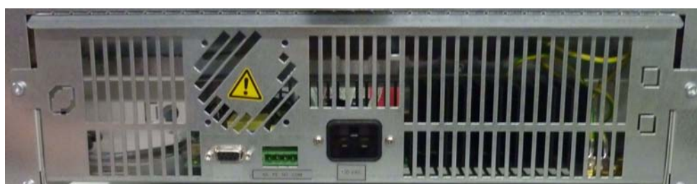
Figure 4-11 Signal Interfaces and Power Socket
