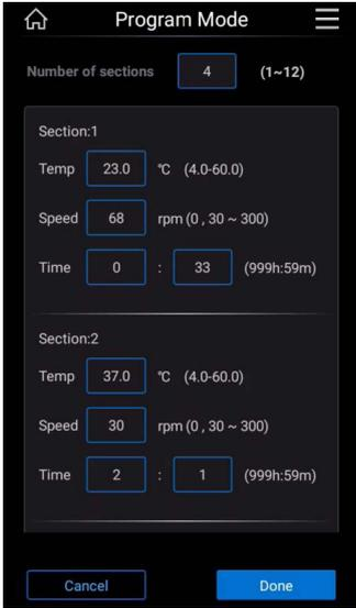
This interface allows for program control mode parameter settings. Set the number of segments at the top of the interface, slide settings in the middle of the interface, and cancel and save operations at the bottom of the interface.
