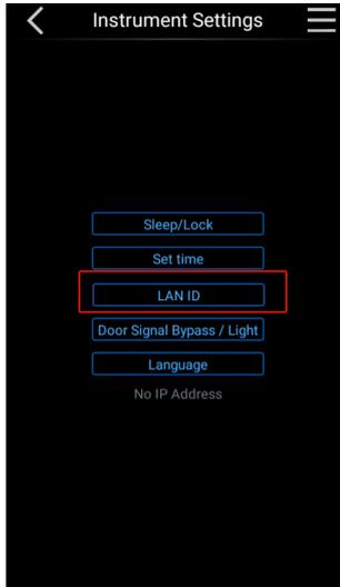
LAN ID and SN code can be set on the interface. LAN ID should be unique for each device, with a maximum of 32 devices can be connected and added here. No restriction for SN code.
