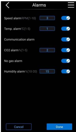
Set speed alarm, temperature alarm, communication alarm, CO2 alarm, no gas alarm and humidity alarm.
