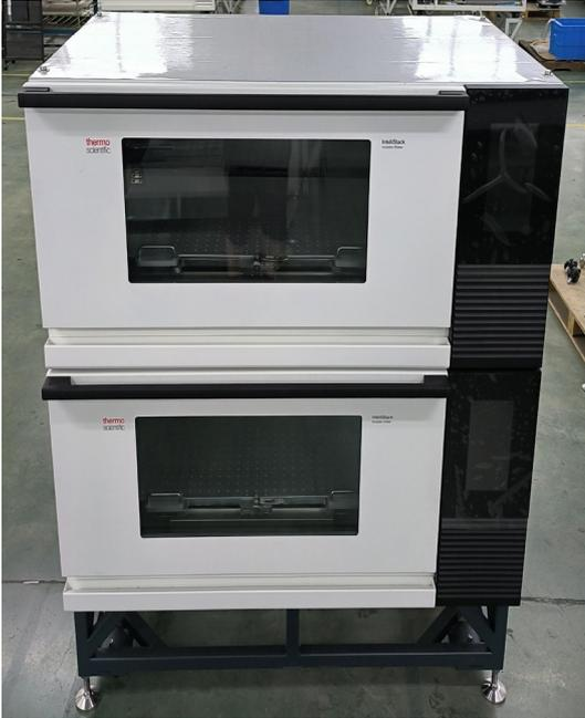
**Note:** The casters are intended for use during positioning of the product and should only be used for moving short distances. Once the unit is installed in its final location, the casters must be removed.
