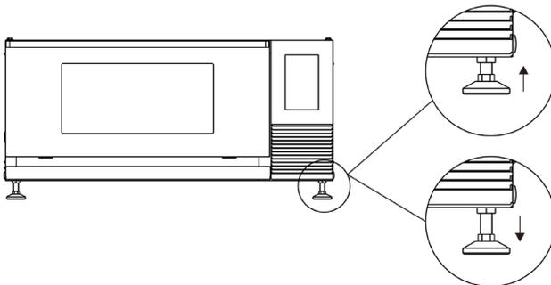
Adjust all feet up to off the ground, the instrument can move on the wheel.
