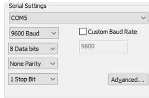
After completing the basic parameter settings, remote monitoring of the device can be completed by combining the Modbus protocol requirements with the provided Modbus address table.
