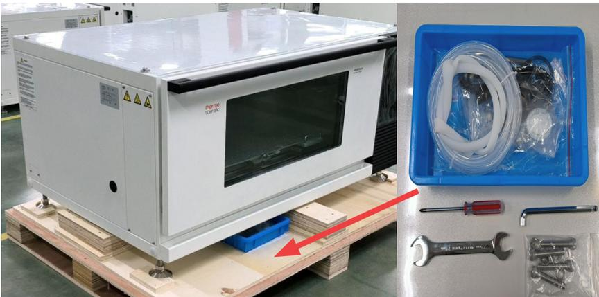
1. The accessories and tools are packed in a blue box, which is usually placed in the gap between the shaker and pallet.
