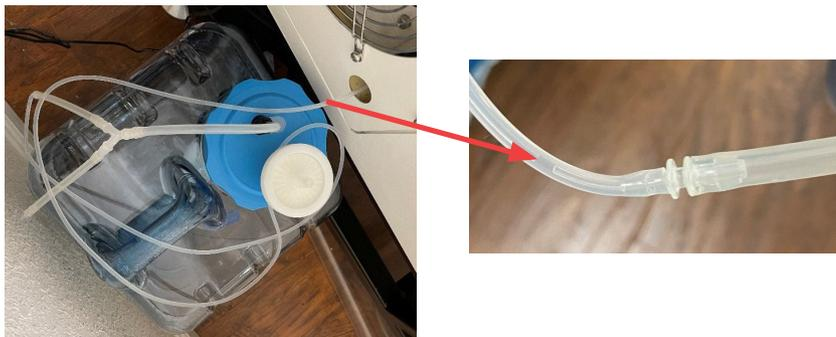
Figure 5: Thin tubing from incubator shaker connected to carboy via 2-way connector
